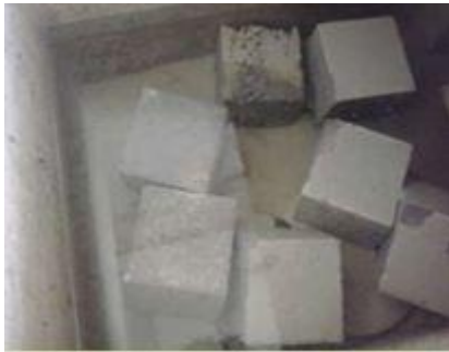
Fig 1 Curing of cubes
